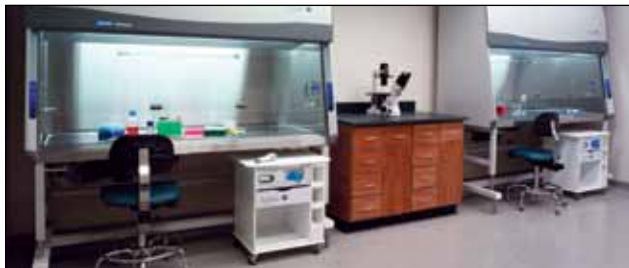
Logic Carts are shown stored beneath two Purifier Logic Biosafety Cabinets on Hydraulic Lift Base Stands.
